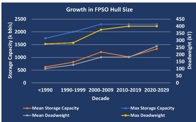
The reasons for this increase are similar to those given above for topsides weight. Larger processing capacities require more storage volume to maintain a reasonable offloading frequency. But the larger and heavier topsides need more deck space and deadweight capacity.
