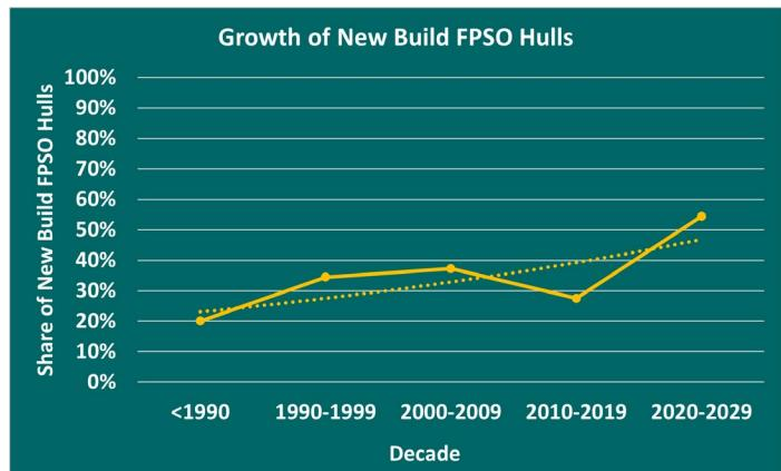
One of the main implications of this move to larger new-build hulls is the risk that project schedules will increase, as they have a longer delivery time than the topsides modules. To mitigate this, the hull can be standardised and ordered in advance of FID, to take it off the critical path. SBM Offshore has done this very successfully with their Fast4Ward programme (Ref 6), and other FPSO contractors are now following this lead (Ref 2, 7).
